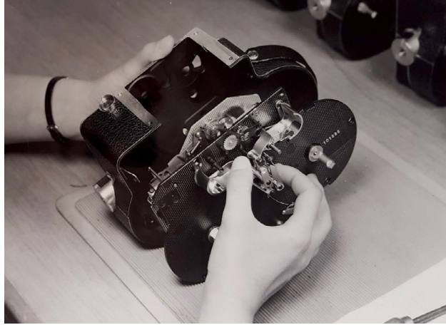
Assembling the shell and mechanism of the H16 camera. See database entry.
